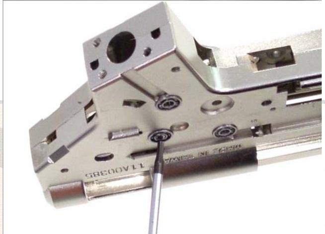
**3:** Put the sector gear in place. Check that the sector gear does not hit the spur gear and does not hit the cut off lever. If the sector gear hits the cut off lever and / or the spur gear, place more shims under the sector gear. Note that the teeth of the sector gear still maintain maximum contact surface with the teeth of the spur gear! Now repeat step 2b with the sector gear.
