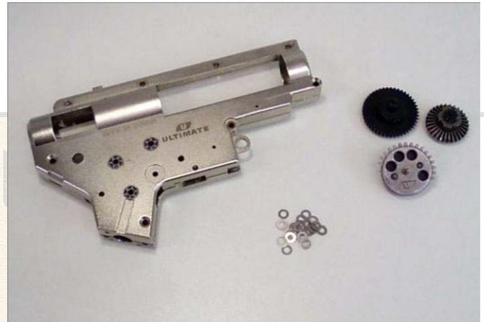
**2a:** Place the spur gear in the gearbox. Make sure that the spur gear has enough space to turn freely from the gearbox. If not, the spur gear will hit the gearbox. This can be seen from a circular sanding spot under the gear, on the gearbox.
