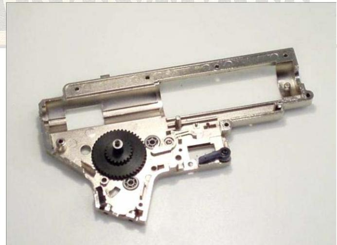
**2b:** Now place the other gearbox half on it. Screw it in with the screws that are around the gears (often 5 or 6 screws). Tighten it properly!
